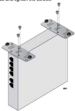
4. Turn the device and place the brackets on the flat surface.
