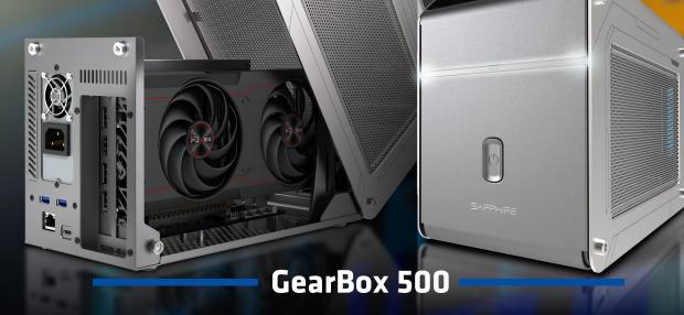
The GearBox 500 Thunderbolt<sup>™</sup> 3 eGFX enclosure enables users to convert a Thunderbolt <sup>™</sup> 3 / 4 Mac or Windows 10 device into a powerful productivity and gaming desktop. The enclosure features a lightning quick 40Gbps Thunderbolt<sup>™</sup> 3 connecting interface that handles various types of data and is capable of charging a Thunderbolt <sup>™</sup> 3 / 4 configured laptop.
