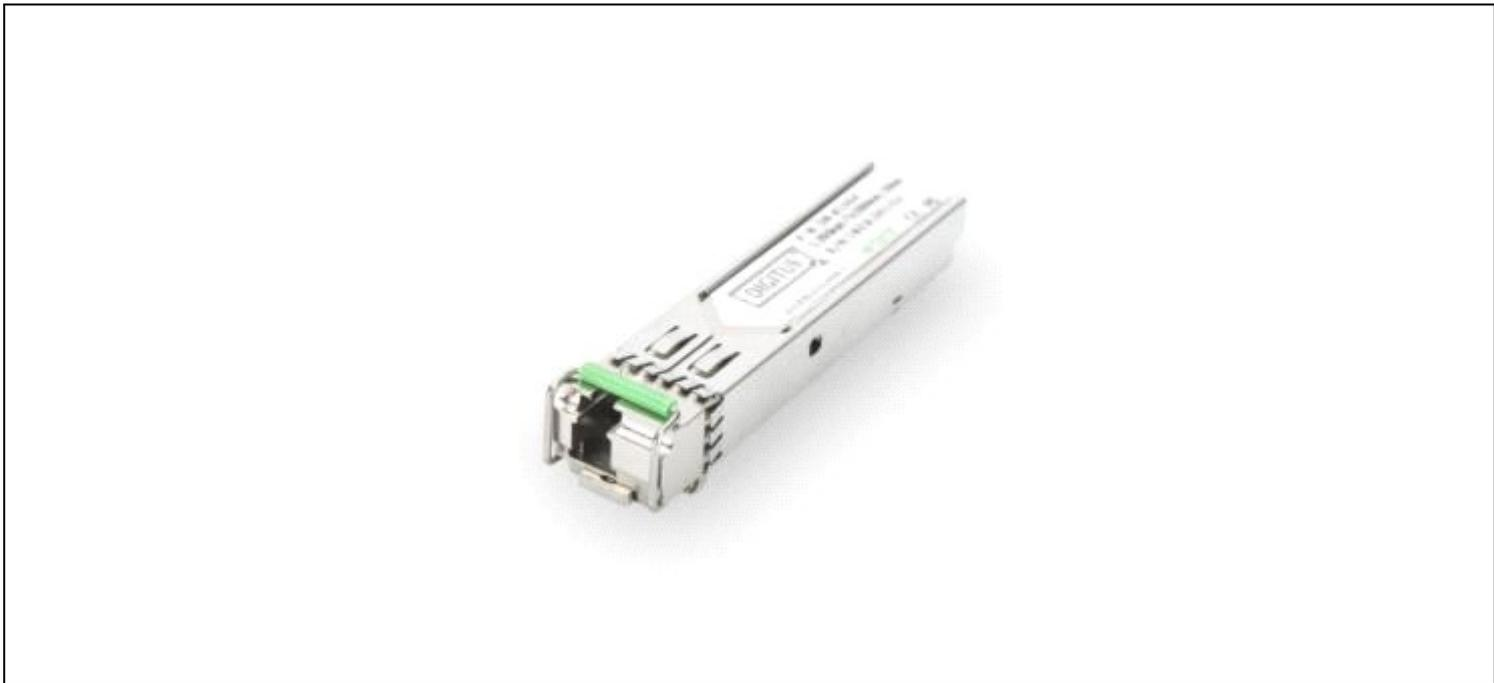
**1.25 Gbps BiDi WDM SFP Module, Up to 20km with DDM support, Singlemode, LC Simplex Connector 1000Base-LX, Tx1550nm/Rx1310nm**
