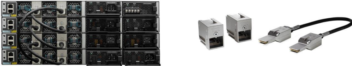
Figure 4. StackWise-160 Kit with Stack Adapters and Cables
