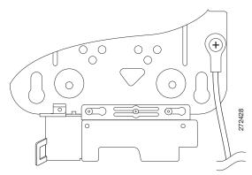
**Step 7** Use a Phillips screwdriver to tighten the ground screw.
