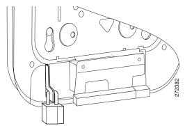
**Step 4** Rotate the padlock into the padlock area. See Figure 13.
